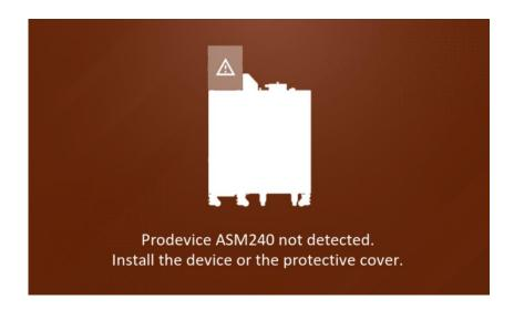
When ASM240 is absent, the safety cover must be installed to operate the shredder. To operate the machine after this message appears on screen, restart the device.
