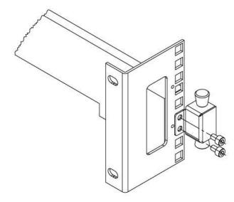
Then, attach the drawer mounting piece to the holes in the drawer body using M4 screws. You can install a long element (1) or a short element (2) depending on the dimensions of your rack cabinet.
