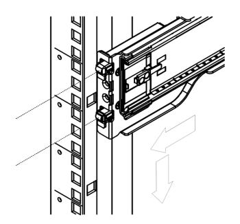
Then, secure the rails to the rack mounting rails using the built-in latches.
