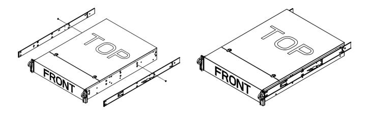
Before starting the installation, make sure that you put the corresponding rails on the left and right sides of the drawer.
